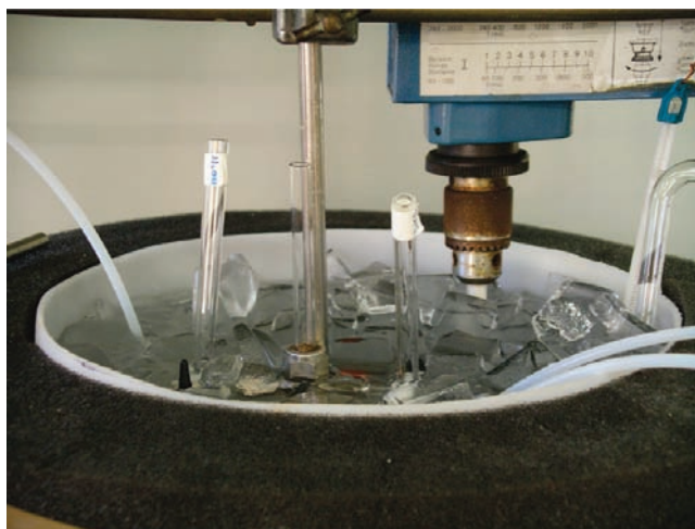
Figure 5. Mixing system in ice–water bath.
