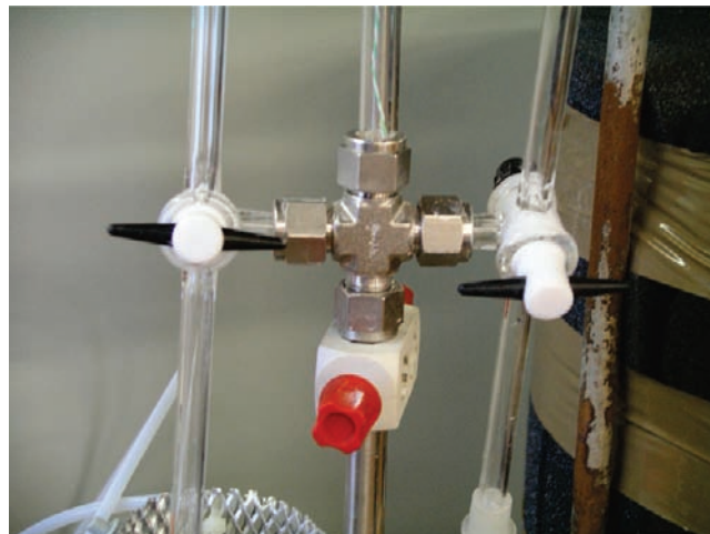
Figure 3. Top of static mixer and inlet system.
