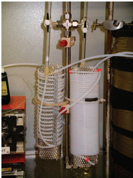
Figure 2. Intercoiled inlet tubes (left), coiled exit tube (9 m, right), static mixer (vertical in centre).
